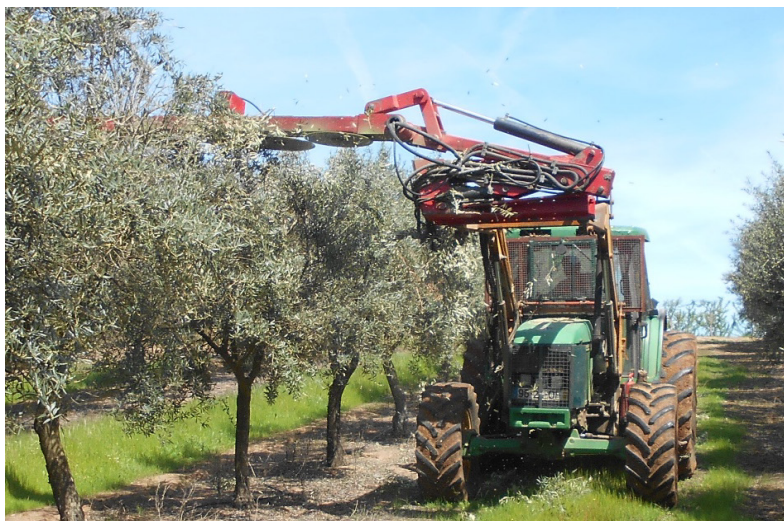
Figure 1. Disc-saw pruning machine performed “topping”.
