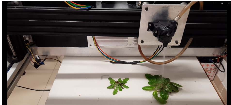
Figure 15. Result of real-time application: positioning of nozzle and spray atomization.
