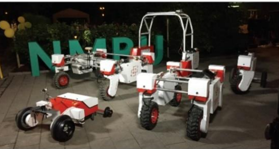
b) Modular robotic system for different agricultural tasks (Grimstad and From 2017).
