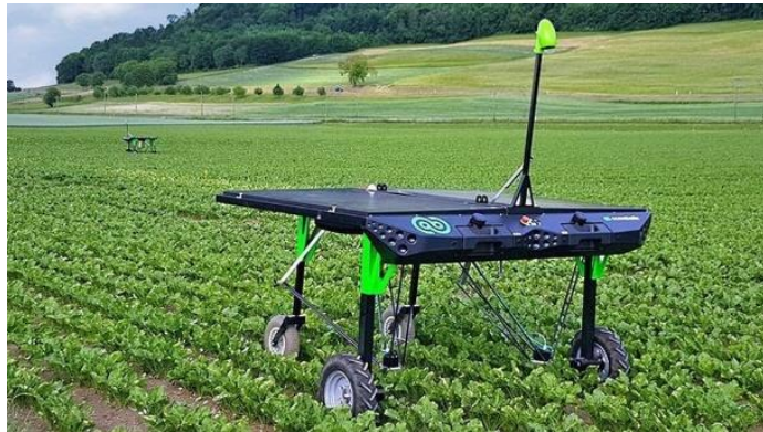
(a) Precision spraying robot ARA (Ecobotix 2019).
