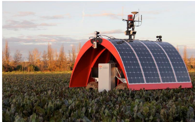
(b) Precision spraying robot Ladybird (Sukkarieh 2016).
