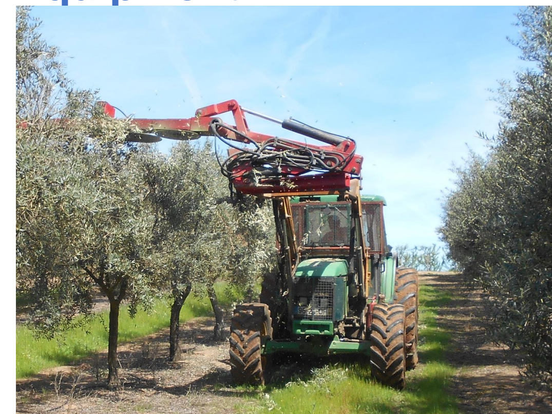
Fig. 1 "Topping" with disc-saw pruning machine
