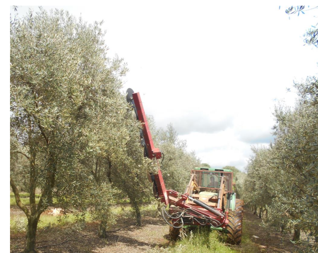
Fig. 2 "Hedging" with disc-saw pruning machine
